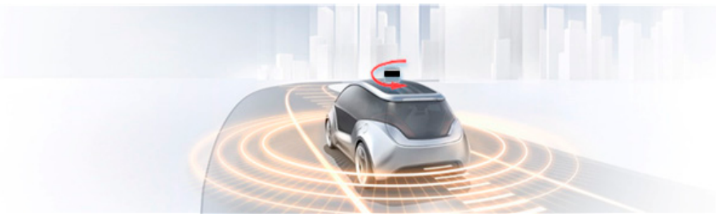
Figure 2. Example of a LiDAR sensor capable of 360° viewing angle working in constant rotation.
