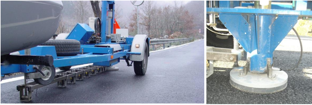
Figure 5. FWD tests: during operation (left); detail of the plate on ISAC base layer (right)
