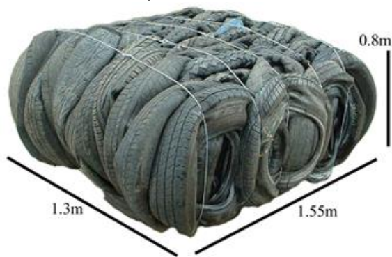
Figure 1. A typical tyre bale with dimensions
