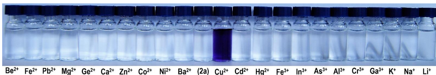
Figure S3. Colour changes observed in acetonitrile solutions of probe 1 ( 1.0 \times 10^{-5} mol L -1 ) upon addition of 10 equiv. of selected metal cations.
