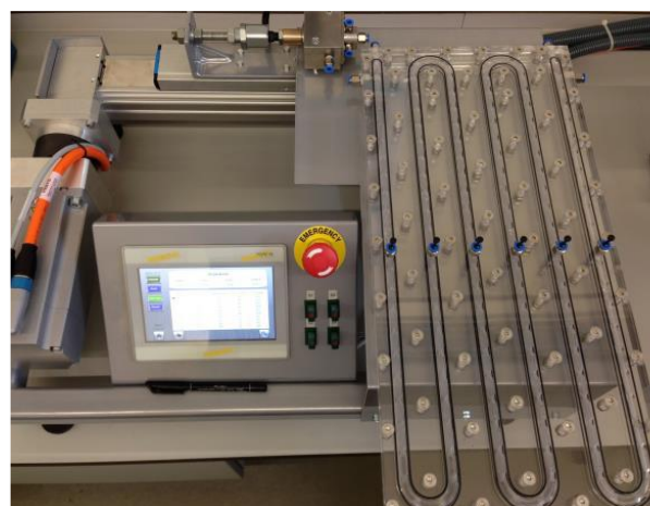
Figure 1. Modular “LEGO” type OFR
