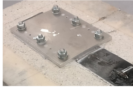
(b) Anchorage Slippage observed at elevated temperature – L100_T150_ET2
