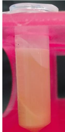
Figure A5. Image of a freeze-dried sample after rehydration and centrifugation. A considerable deposit of particles that had not undergone a properly rehydration is showed.
