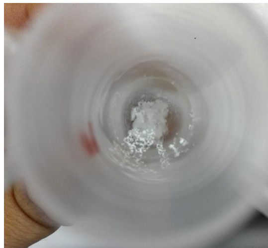
Figure A6. Image of a nanospray-dried sample after rehydration in phosphate buffer and submission to sonication. Is visible a remaining suspension containing some macroaggregates as well as some deposit of powder.
