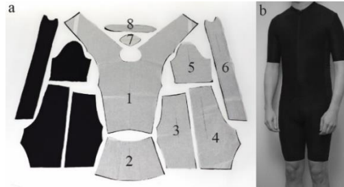
Fig. 3. Garment prototype: a) Patterns cut (1) torso; 2) back pocket; 3) front leg; 4) back leg; 5) sleeve; 6) side yoke; 7) crotch yoke; 8) collar); b) fitting
