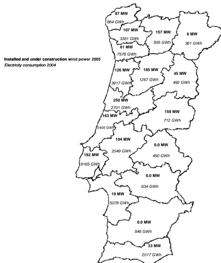
Figure 6- Installed wind power in Portugal (excluding islands). Sources: INEGI (2005) and DGGE site.
