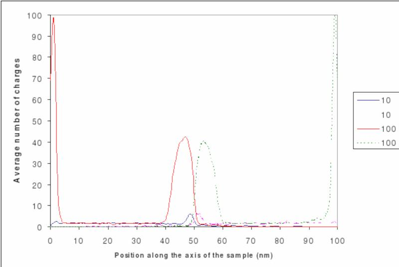
Average number of charges along the axis of the sample, for two dielectric constants of the nanoparticle (10 and 100), embedded in a sample of type D. Solid lines represent electrons and dashed
