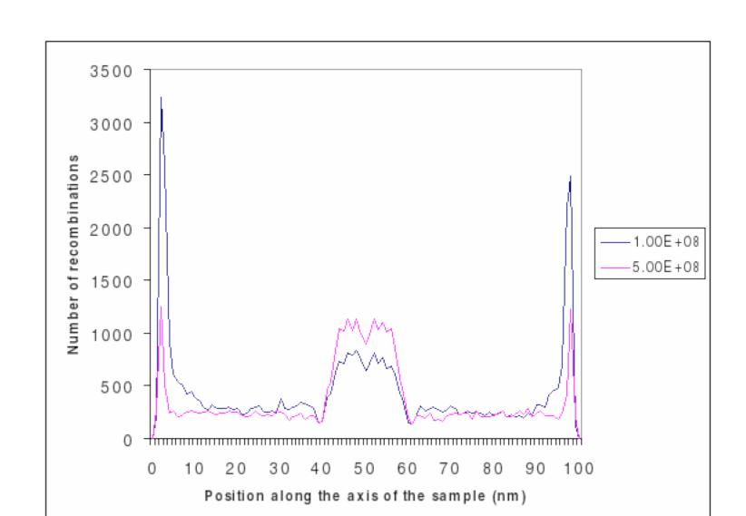
Number of recombinations as a function of the position in the sample, for sample ABA, for applied electric fields of 10<sup>8</sup> V/m and 5x10<sup>8</sup> V/m.
