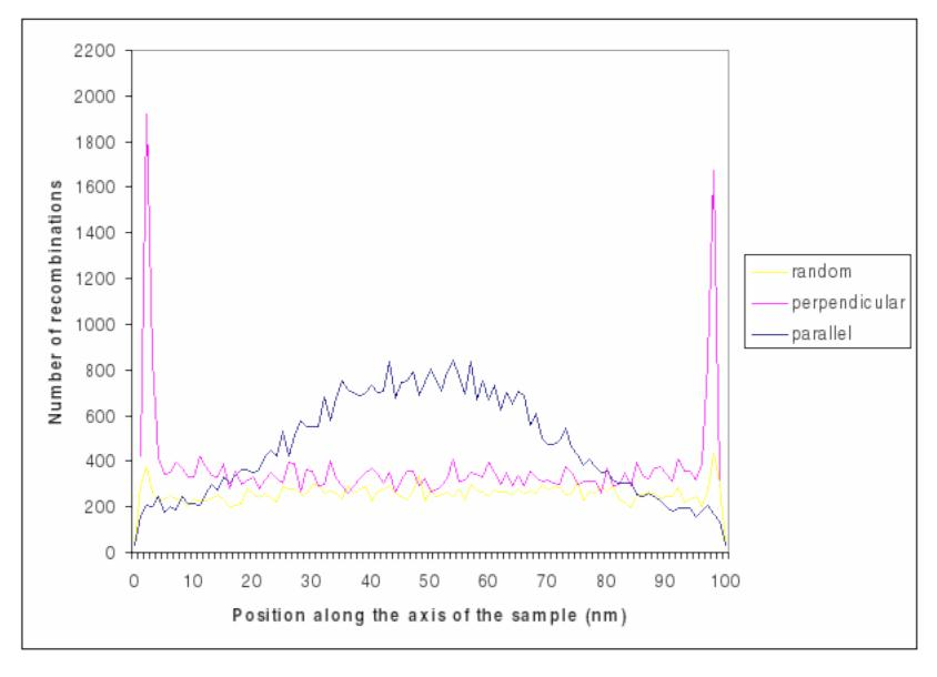
Number of recombinations as a function of the position in the sample, for three different types of samples, for an applied electric field of 5x10<sup>8</sup> V/m.
