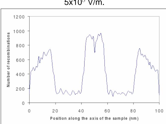
Number of recombinations as a function of the position in the sample, for sample BABAB, for an applied electric field of 5x10<sup>8</sup> V/m.
