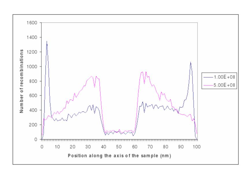
Number of recombinations as a function of the position in the sample, for sample BAB, for applied electric fields of 10<sup>8</sup> V/m and 5x10<sup>8</sup> V/m.
