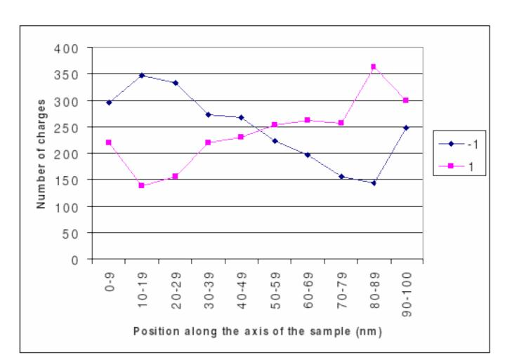
Number of charges (both positive and negative) as a function of the position in the sample, for samples of type A, after 2500 iterations.
