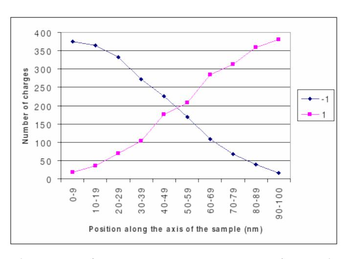
Number of charges (both positive and negative) as a function of the position in the sample, for samples of type B, after 2500 iterations.
