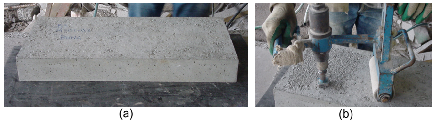
Figure 1 The top surface of one specimen before roughing (a) and the rough machine (b).
