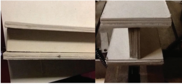
Figure 10. Relative displacement on a beam after bending test.
