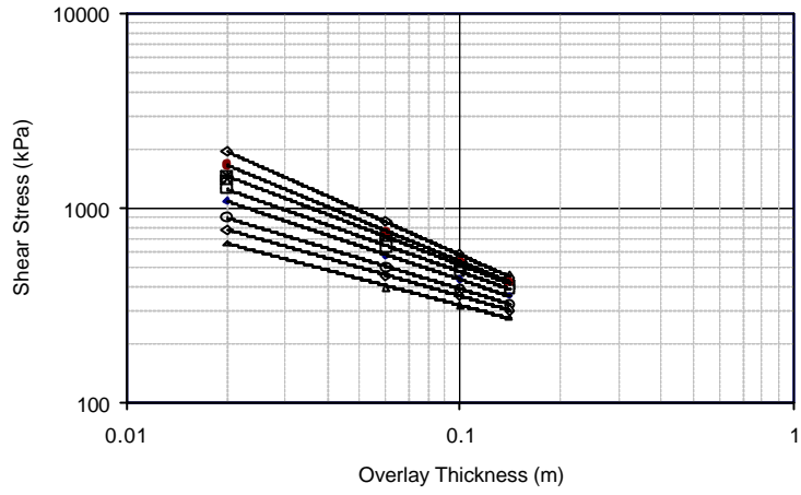
Figure 3. Typical influence of the overlay thickness on shear stress in the zone above crack
