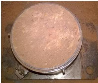
Figura 22- Molde Proctor rasado
