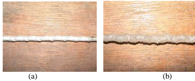
Figure 2 – Rib structure (a) braided fabric (b) braided reinforced composite rod
