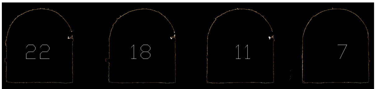
Figure 37. Damage profiles from clouds of points for Zone C
