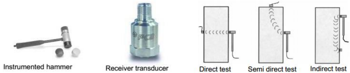
Figure 12. Sonic testing elements (Ramos & Lourenço, 2016)
