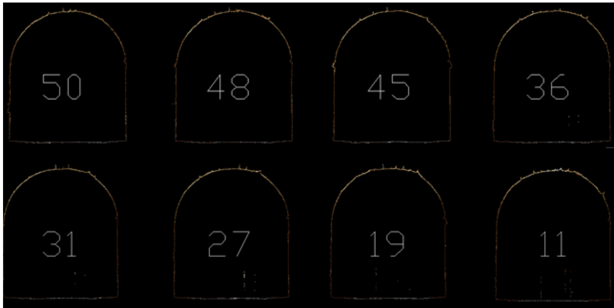
Figure 36. Damage profiles from clouds of points for Zone B
