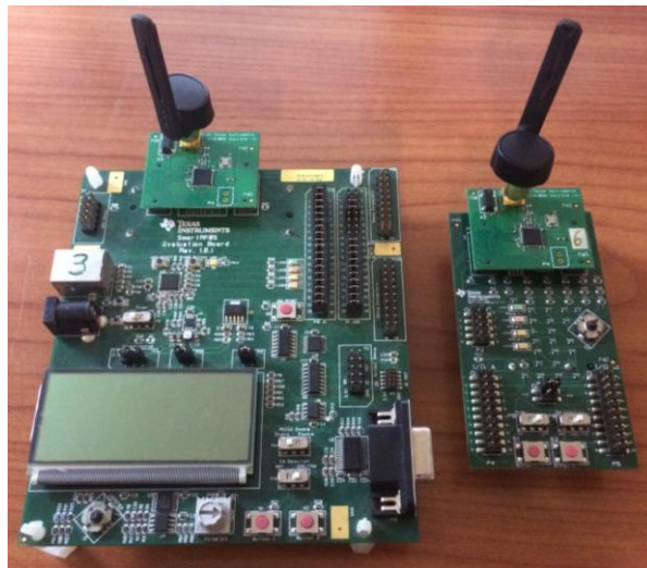
Figure 4.1: CC2530 development board (left) and battery board (right) with evaluation modules.
