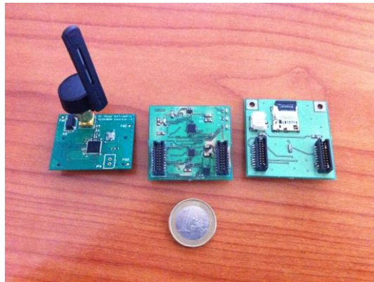
Figure 5.1: Sensor node prototype. The CC2530 module is shown on the left, the sensor and battery board in the middle and the SDC board on the right.
