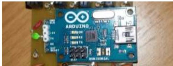
Figura 42 - *Arduino USB Serial Light Adapter*
