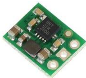
Figura 64 - Conversor step-up U1V10F5 da Pololu [58].
