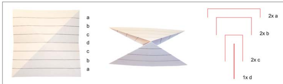
Figure 6. Waterbomb model open and closed (left and centre); SMA shapes (right)
