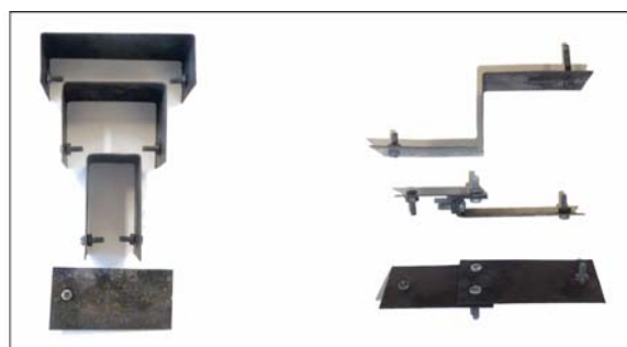
Figure 8. Waterbomb dies (left); Squaretwist dies (right)
