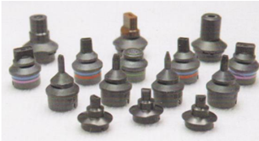
Figura 31: Pipetes de coleta de material (ASM)
