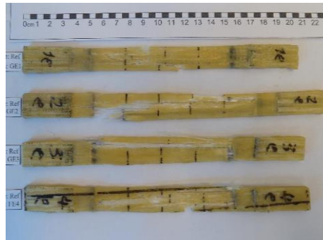
Figure 4. Typical failure mode of GFRP coupons
