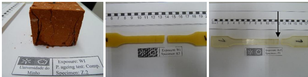
Figure 3. Typical failure mode of brick, epoxy resin and primer
