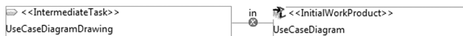
Figure 58 – An example of a validation error in the constraint on the relation between intermediate tasks and work products.
