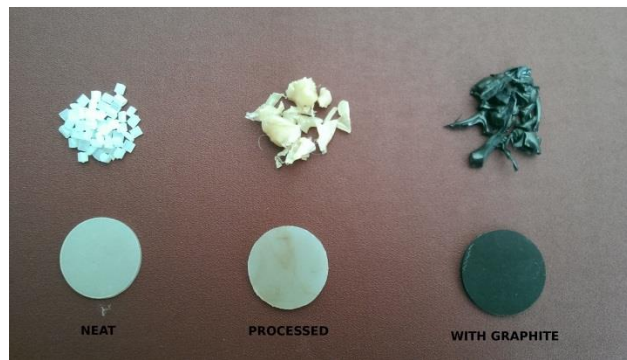
Figure 8. Material from which the disks were made and their final shape after molding. From left to right, neat (Ultramid®), processed (Ultramid®) and nanocomposite.
