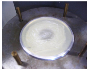
Fig.7 - Cream film applied manually to the lower support base of the silicone rubber
