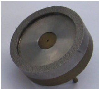
Fig.2 - Metallic (ring type) upper body used in previous FRICTORQ fabric tests
