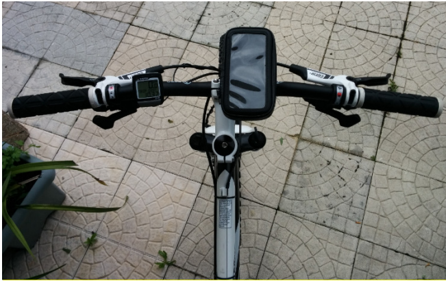
Fig. 5. Placement of the smartphone for the roughness test.
