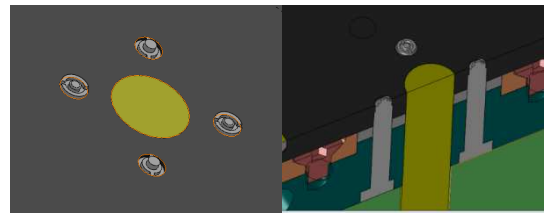
Figure 6. CAD drawing of the moulding cavities and the central ejector pin in detail.
