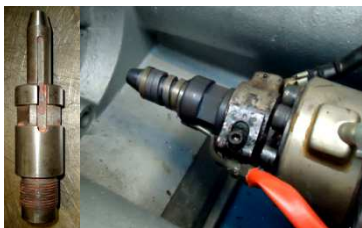
Figure 8. Machined injection nozzle in steel 2343.
