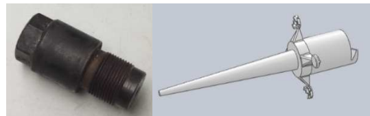
Figure 10. Standard nozzle on the left; sprue and runner system on the right.
