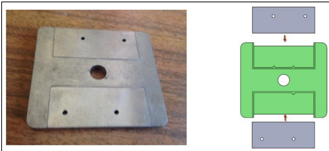
Figure 35 – Back view of the cavity insert after manufacturing and with closed compartment (left) and before manufacturing and with open compartment (right).
