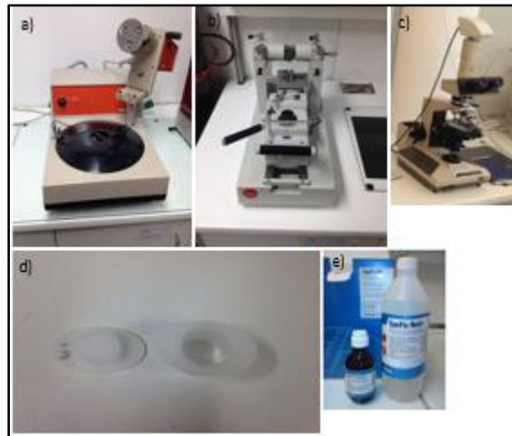
Figure 42 – Equipments and accessories needed to optical characterization: a) polish machine; b) microtome; c) Olympus transmission microscope; d) plastic mold used; e) Resin and hardener (Epofix kit).
