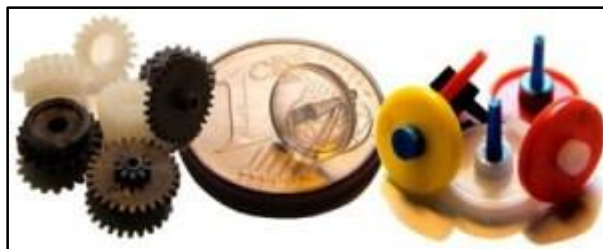
Figure 2 – Examples of microinjection molding parts with one component (left) and two components (right). [13]
