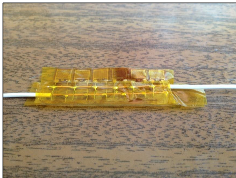
Figure 38 – System of strain gages connect in parallel by copper wires.
