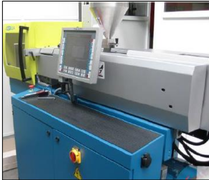
Figure 31 – Boy 12A micro-injection machine.
