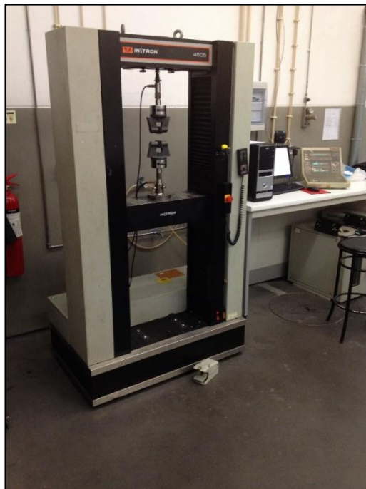
Figure 48 – Instron 4505 strength testing machine.
