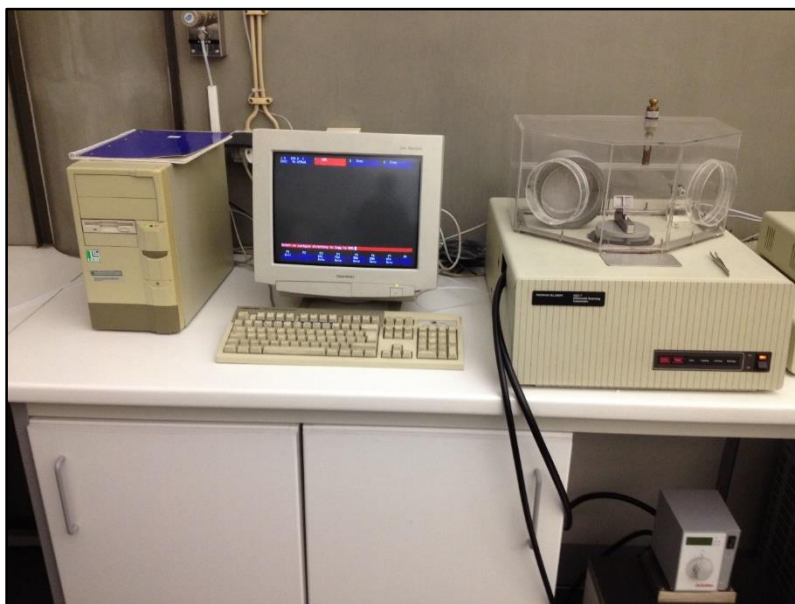
Figure 53 – DSC 7 produced by Perkin Elmer.
