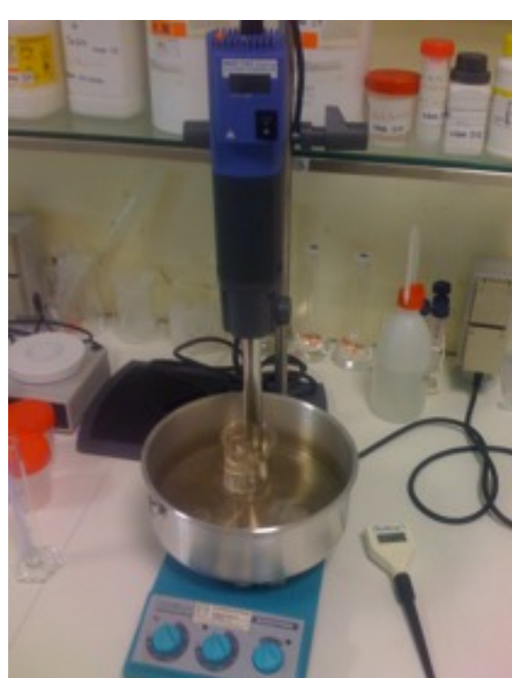
Figure 1. Experimental setup utilized for the preparation of lipid nanovesicles encasing T4-bacteriophages.
