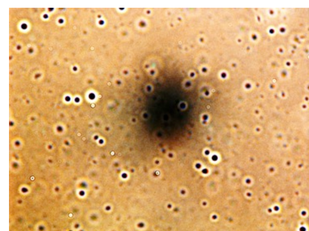
Figure 2. Physical appearance of the lipid nanovesicles (Water-in-Oil-in-Water multiple nanoemulsion), as observed under an optical microscope at maximum resolution (x100).
