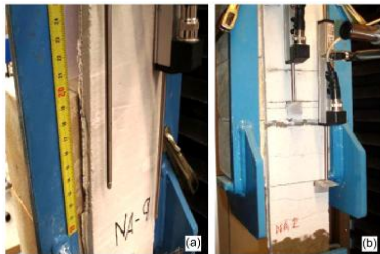
Fig. 8 Failure modes in BTRM specimens: debonding at the substrate-matrix interface in specimens with anchorage length of 85 mm (a) and slipping of the fibre rovings from the matrix in specimens with anchorage length of 220 mm (b)
