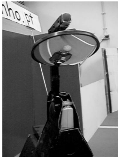
Fig. 2. (a) Omni-directional catadioptric vision system consisting of a camera and a parabolic mirror; (b) an image taken by a conical-spherical sensor.
