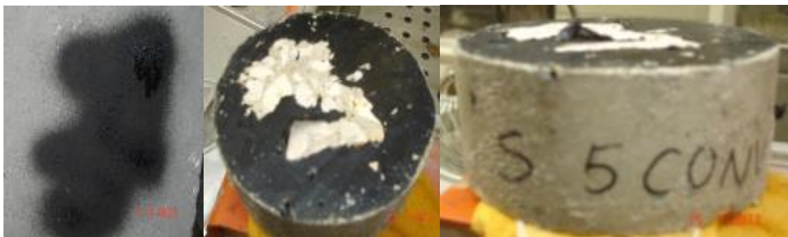
Figure 5 - Removal process of spray paint concrete surface with sacrificial protection AGS 2
