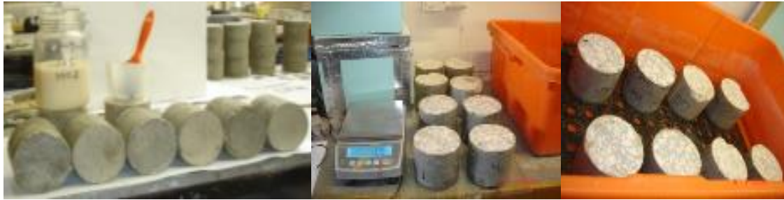
Figure 7- Procedures of water absorption by capillarity test
