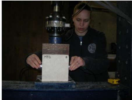
Figure 10. Mortar block test setup including positioning of ultrasonic sensors
