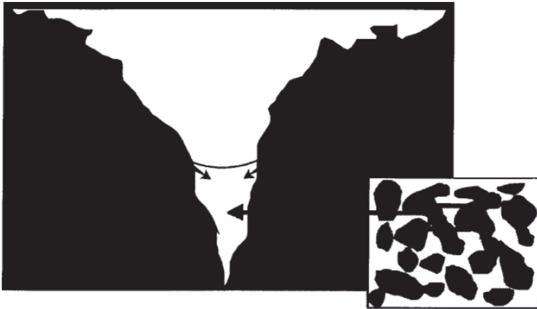
Figure 2.10 – Effect of pore meniscus and surface tension on the drying shrinkage of mortar (Balogh, 1996)
