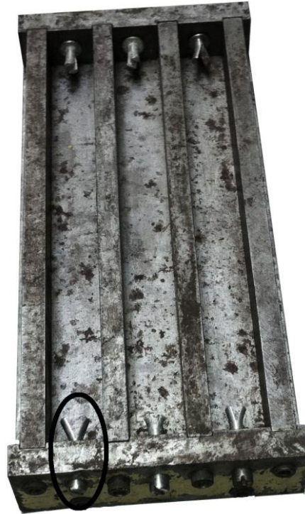
Figure 4.6 – Detail of the plug embedded in each extremity of the specimen
