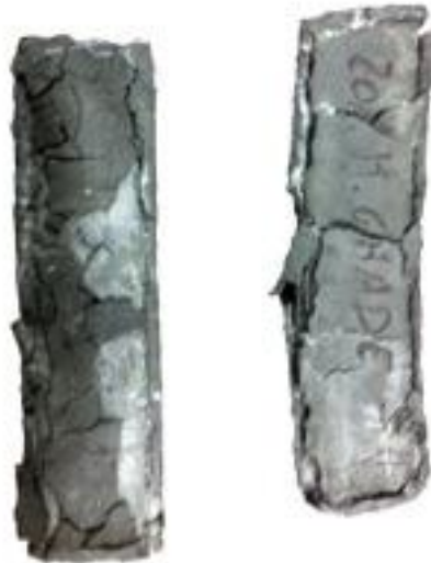
Figure 4.3 - Photo of specimens from mixtures 5 and 7 upon unmoulding after 20h
