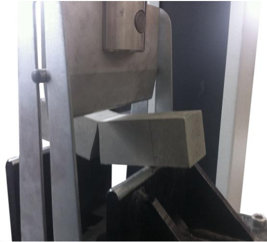
Figure 4.4 - Two halves of the specimen to be used for compressive strength testing after the flexural strength procedure
