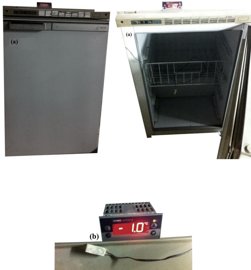
Figure 4.13 – Deepfreeze used (a) and detail of thermostat with the probe (b)
