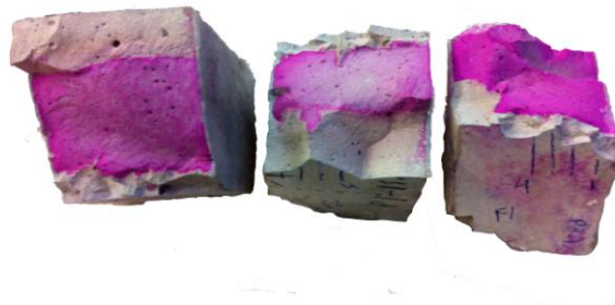
Figure 5.13 – Specimen appearance after vaporization of phenolphthalein solution
