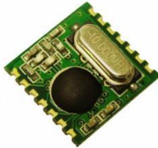
Figura 2-9-Alpha RF Transceiver [3]
