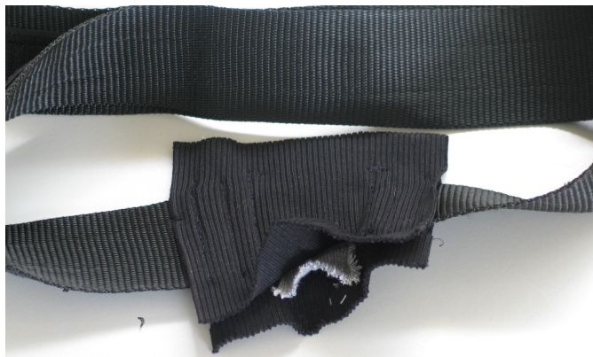
Fig. 8. Breathing movement measurement accessory based on electrically conductive knitted fabric.
