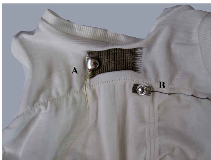
Fig. 1. Textile electrode embedded - knitted directly - into a shirt fabric (A) and electrical path to the electrode also embedded in the knitted fabric (B).
