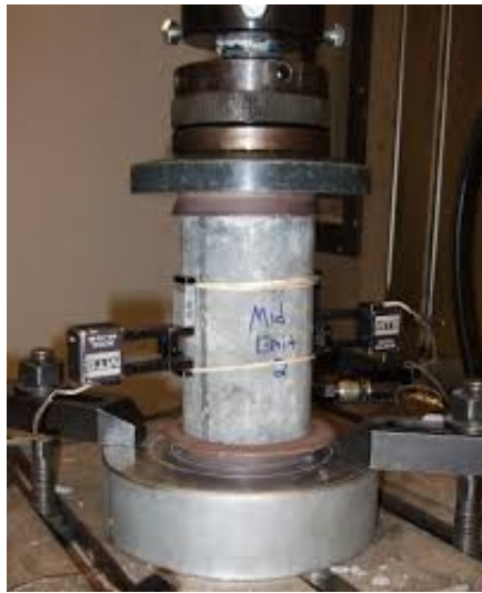
Figure 2.29: Compression testing on a concrete specimen [17]
