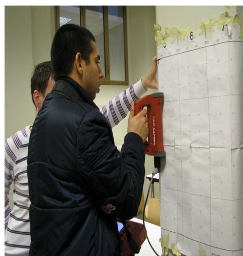
Figure 2.10: Testing of wall by ferroskan [2]
