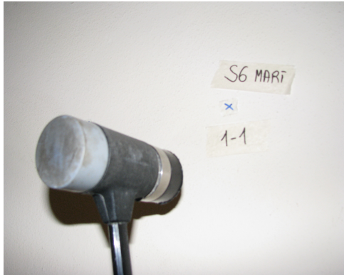
Figure 2.2: Hammer to generate pulse for sonic test [2]
