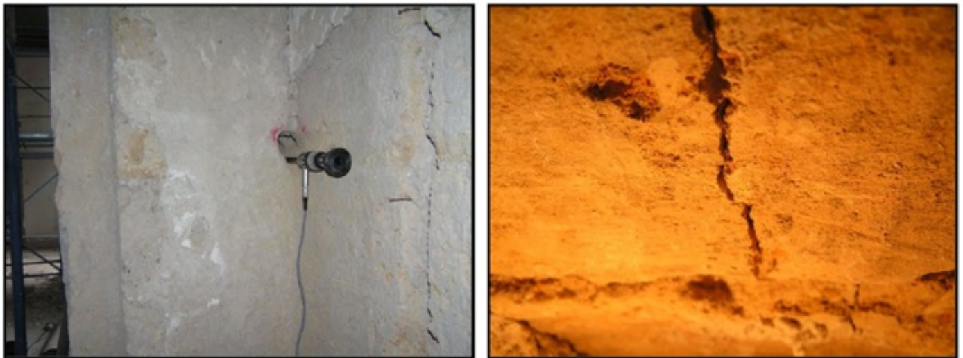
Figure 2.28: Execution of endoscopic investigation (left) and its endoscopic picture (right) [16]
