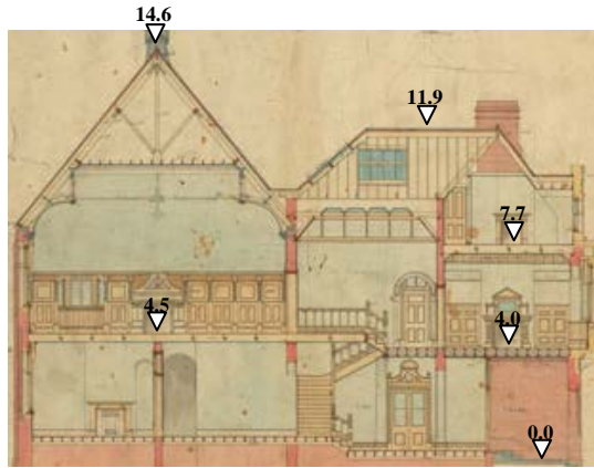
FIGURE 3 Horizontal view of East elevation and section from South (original drawings by Samuel Hurst Seager, ca. 1886).
