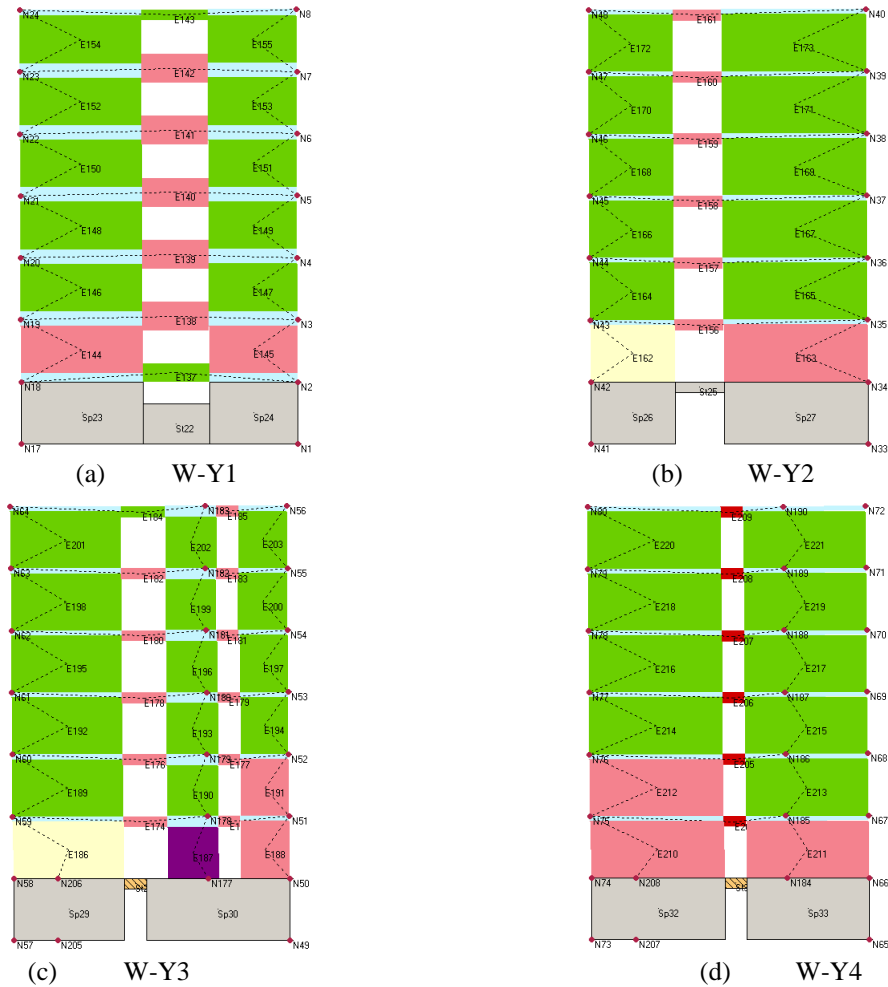
Figure 7.8 - Damage levels according to software 3Muri
