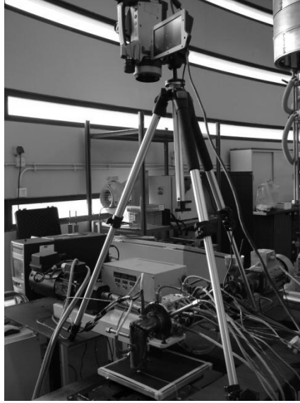
Figure 5.4 – Position of the thermo graphic camera to measure the temperature evolution of the deposited material.
