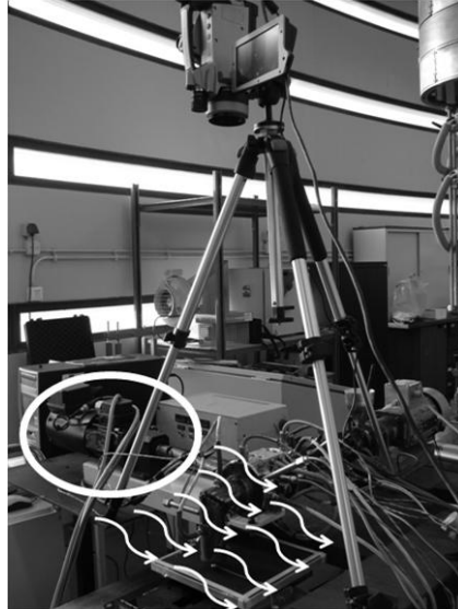
Figure 5.5 – Air movement occurring in the surrounding of the 3D table.
