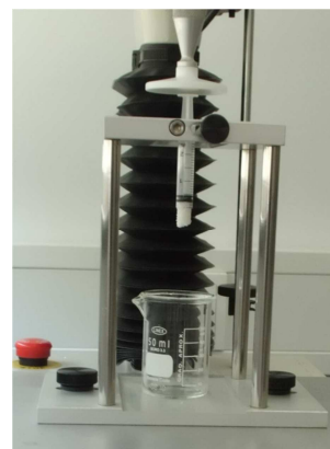
Figure 2.1: Syringe with the injectable system on the texture analyzer.
