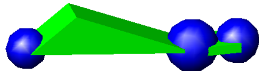
Fig. 2 Foot geometry with identification of the spheres position used in the contact model
