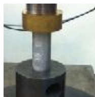
Figure 6 – Disposition of uniform metal foam in compression test
