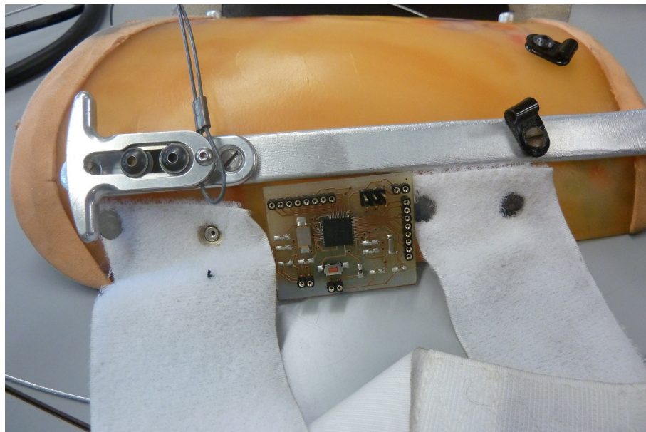
Figure 5.20: Installed microcontroller board
