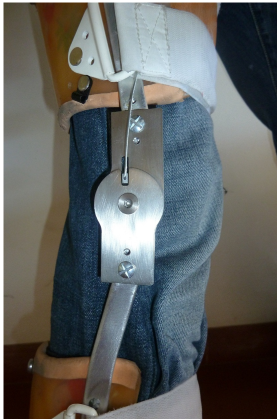
Figure 5.9: KAFO with the built mechanism
