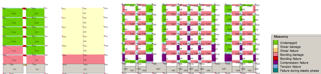
Figure 13. Damage in the walls in "+Y" direction at the failure stage: (a) W-Y4; (b) W-Y6; (c) W-X1; (d) legend.
