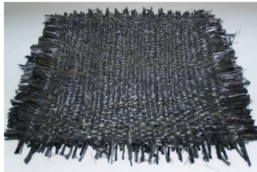
Fig. 11. Primospire ® /carbon woven fabric.
