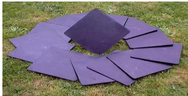
Fig. 10. GF/PP LFT plates made from towpregs
