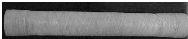
Fig. 8. Filament wound GF/PVC pipe
