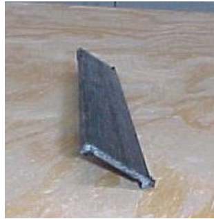
Fig. 9. U-Shape GF/PP pultruded profile made from towpregs
