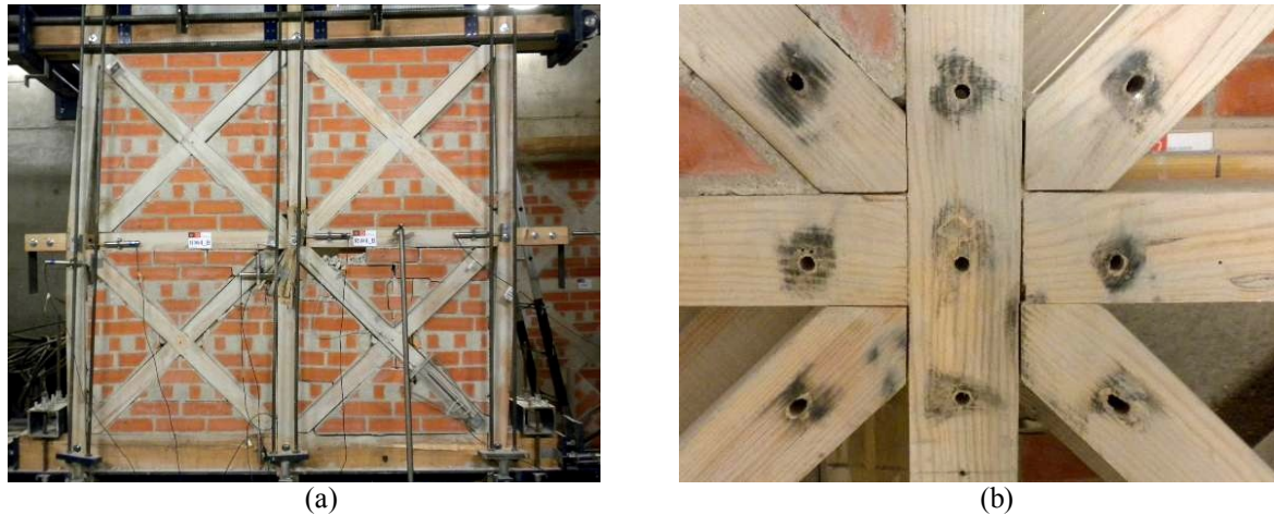
Fig. 11 Typical damages in strengthened walls: (a) shear failure in RIW4_B; (b) holes in RIW2_P deformed becoming oval
