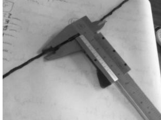
Figure 29. Measurement of the diameter with Vernier caliper..
