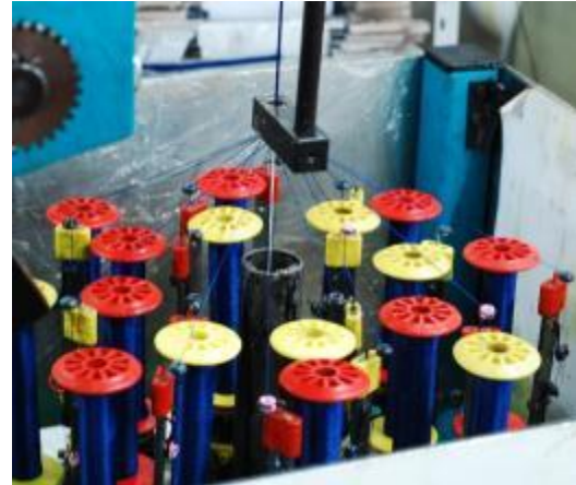
Figure 25. Detail of the braiding process.
