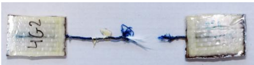
Figure 40. Example of broken sample. The sliding of the fibres is not noticeable at first glance.
