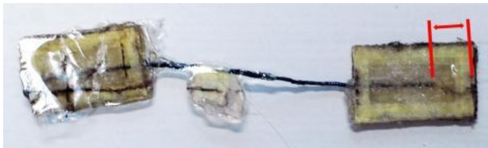
Figure 41. Other type of failing: the whole rod slides into the composite plates.
