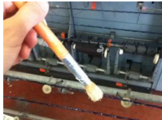
Figure 27. Manual application of polyester resin.
