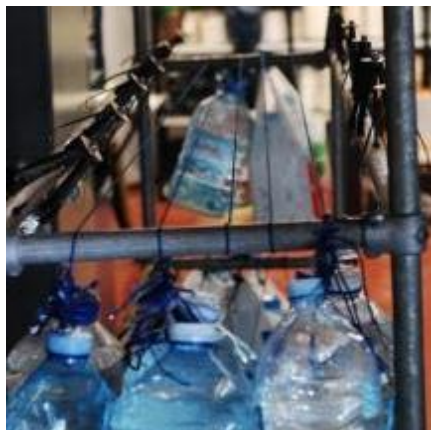
Figure 26. Tensioning of the produced material.
