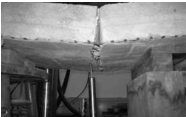
Figure 19. Failure by deep cracking and crushing of brick. [50]
