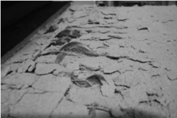
Figure 21. Slipping of the fibres within the mortar matrix [49].
