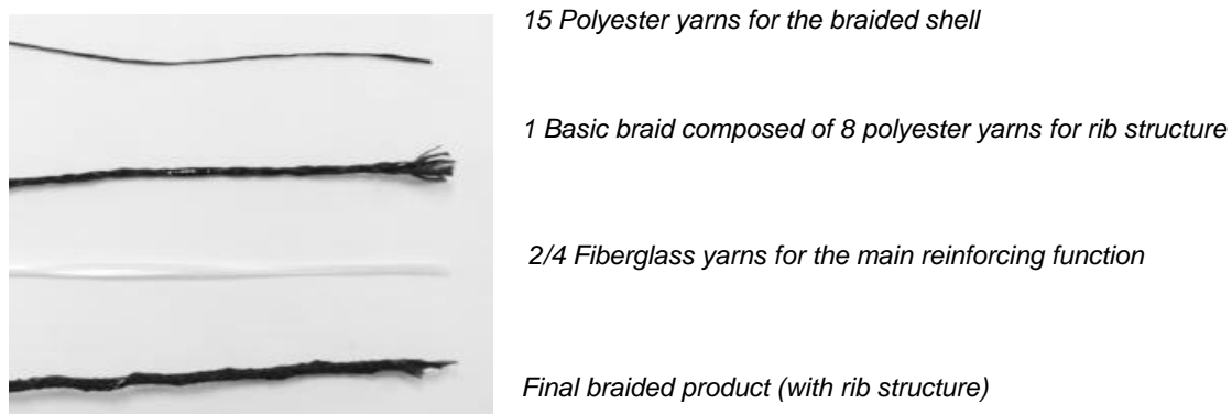
Figure 23. Materials used in the manufacture of the braided retrofitting materials:
