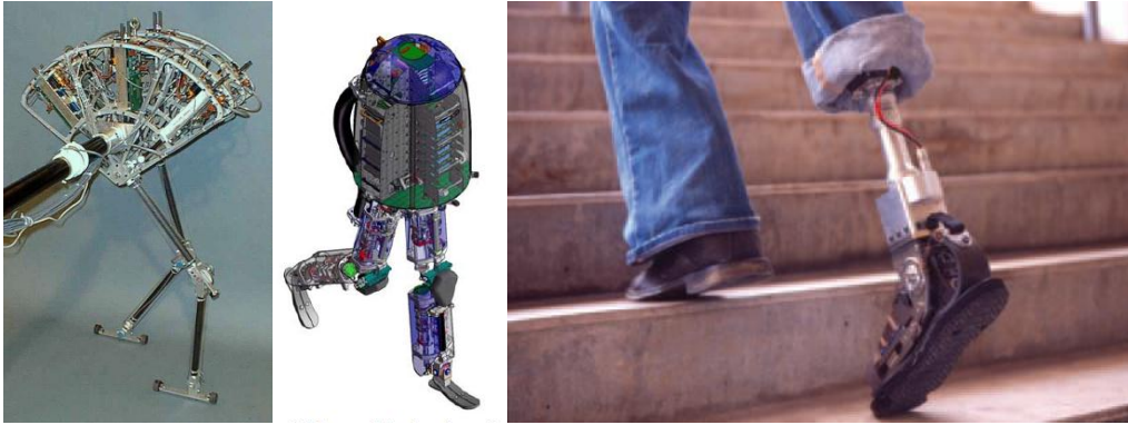
Figure 2.10 | Examples of SEA application. Spring flange [30], M2V2 biped [30] and ankle-foot prosthesis [31] respectively
