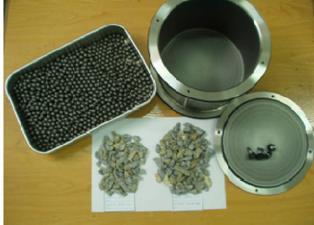
Figure 2. Micro-Deval test equipment
