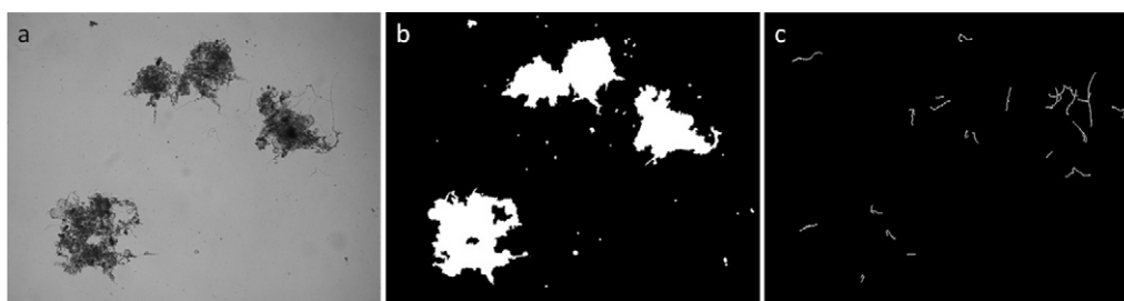
Fig. 1. Bright field image processing: (a) original image, (b) aggregates binary image and (c) filaments binary image.
